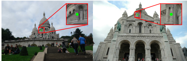
Figure 1. Relative depth from scale. The relative scale of regions around corresponding keypoints is inversely proportional to the relative depth. In this paper we leverage this fact for relative camera pose estimation.
